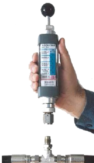
On-line low pressure check
